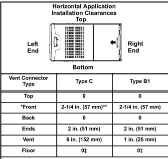
\*Front clearance in alcove installation must be 24 in. (610 mm). Maintain a minimum of 24 in. (610 mm) for front service access. \*\* 4-1/2 in. if single wall vent pipe is used.
